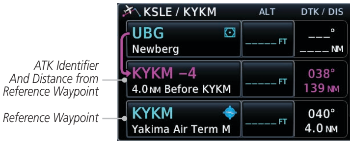
Figure 4-15 ATK Inserted Before Reference Waypoint
