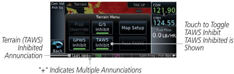
Figure 10-43 TAWS-A Alerting Disabled (TAWS Inhibited) Annunciation
