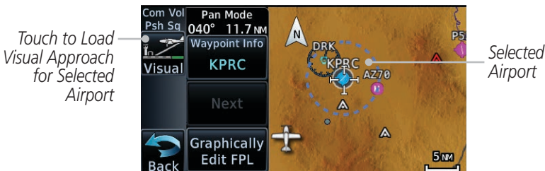
Figure 6-26 Visual Approach Key When Selecting Airport
