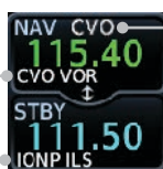
Figure 3-29 Automatic Nav Frequency Ident Decoding
