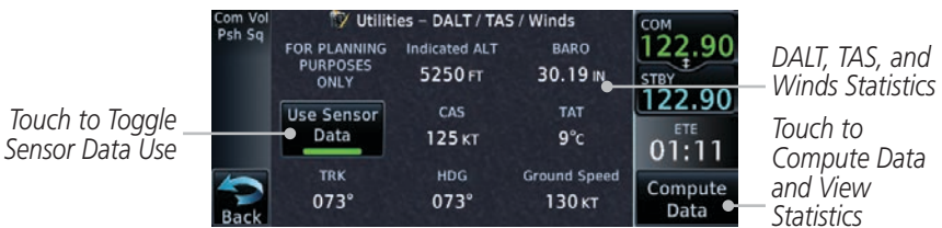
Figure 14-38 Utility DALT/TAS/Winds Page Using Sensor Data and Indicated Altitude
