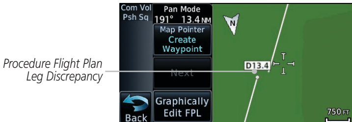
Figure 4-19 Procedure Flight Plan Leg Position Difference
