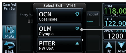
Figure 4-24 Select an Exit Waypoint for the Airway
