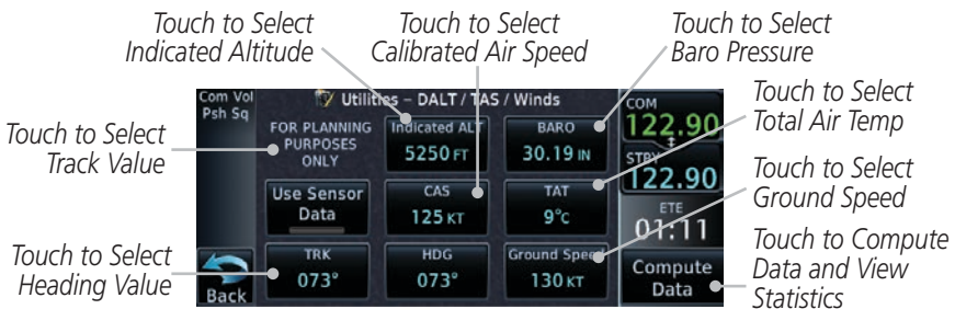
Figure 14-39 Utility DALT/TAS/Winds Page Using Manually Entered Data
