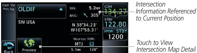
Figure 12-7 Nearest Intersection Waypoint Detail
