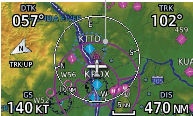
Figure 8-29 Display of Smart Airspaces (Airspace Borders Grayed)
