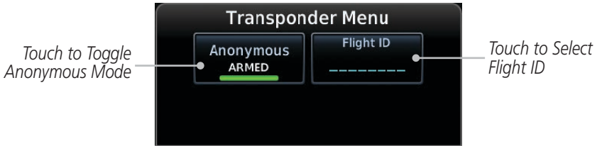
Figure 2-14 ADS-B/Transponder Control Panel
